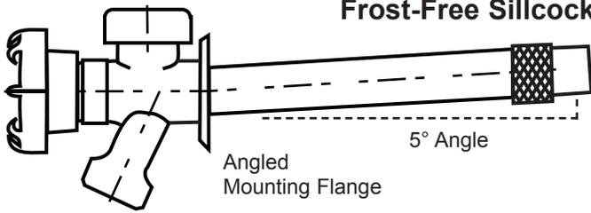
The T-550 is certified to **ASSE 1019 Type A**. In accordance with Sections 1.2.3 and 1.2.4 of this standard, the T-550's operating pressure shall not exceed 125 psi and the operating temperature range is 33 degrees F to 140 degrees F. **SEE INSTALLATION DIAGRAM.**
